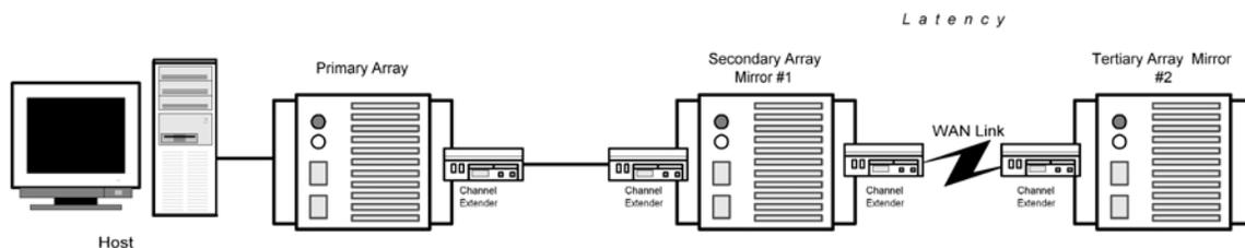
If arrays are mirrored asymmetrically and the time difference between them exceeds a few minutes, it is likely that tape will still play a role in the solution. DR personnel will need to use tape to copy the data that is “out-of-sync” between the arrays, and must carry those backups to the recovery site to bring datasets to a current state.
